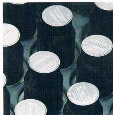
Batches of identical dies can strike many coins at one time.
