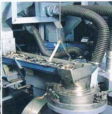
The upsetting mill forms a rim on each blank coin.
