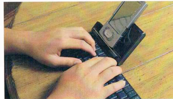
Personal digital assistants, or PDAs, are handheld microcomputers that use either a stylus and touch screen or a tiny keyboard for input.
