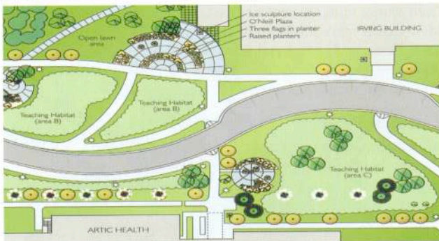
A landscape plan shows the location of trees, shrubs, flower beds, lawns, and walkways.
