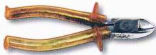
Cutting pliers, which cut either flush or diagonally, are for cutting wires and trimming leads you have soldered.
