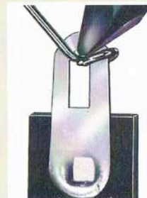
Heat the wire and the lug.
