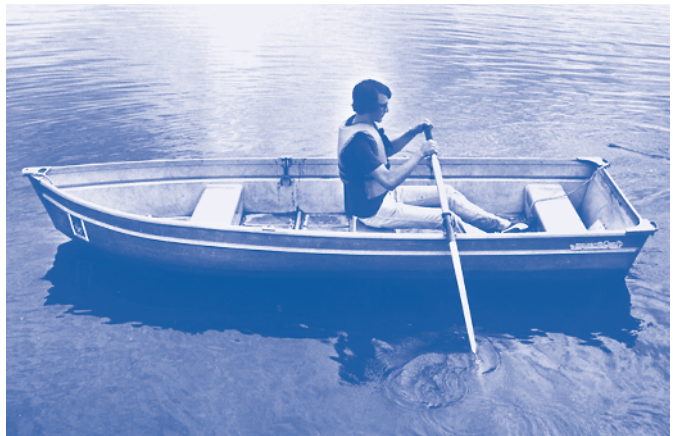
A correctly trimmed boat with single oarsman aboard
