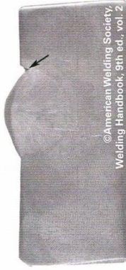
Undercut at the toe of an oxy-fuel arc weld
